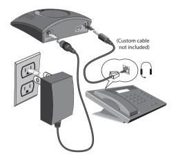
FIGURE 5.0 Connecting Chat 50 to a telephone
